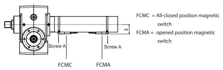
Stroke adjustoment shall be done in following steps, acting on switches "FCMA" and FCMC" as follows:
