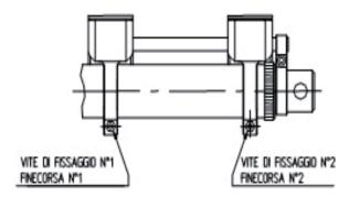
To regulate the stroke of the thrust rodaccording to the required values, act on micro switch 1 and 2 as follows:
