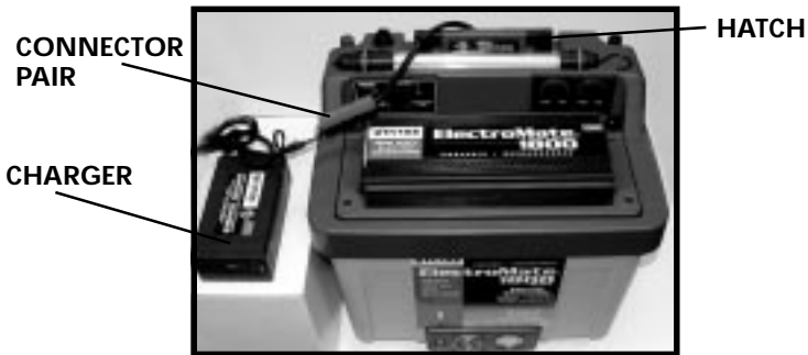
FIGURE 8 – BATTERY CHARGER HOOKED TO ELECTROMATE
