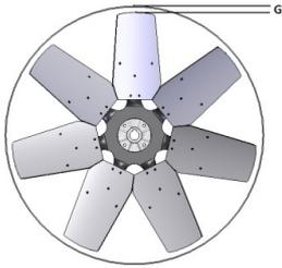
Verify that the distance G, between the impeller and fixed parts, is constant so to avoid impeller frictions
