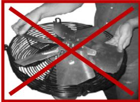
Handle fans with their original packaging. Tools for moving shall be chosen according to the weight and typology of the materials to be moved (form, kind of package, etc..).
