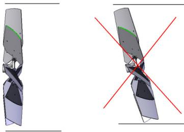
Verify that the fixing position of the fans is suitable to maintain the impeller aligned with the fixed parts
