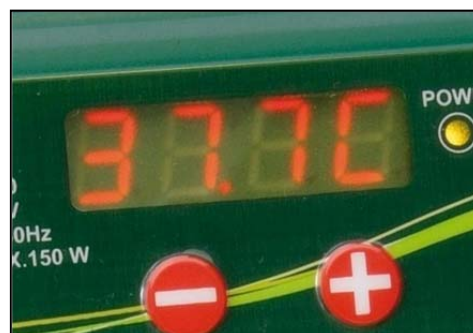
Display with present internal temperature (temperature followed by "C")
