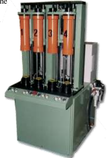
air testing for oil filters
