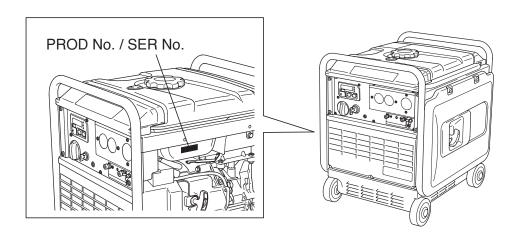
NOTE: When inquiring about your generator or ordering spare parts, always give us the Model, Serial Number and Production Number.
