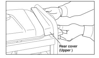
(2) Install the Muffler Cover (Rear) onto the Rear Cover (Upper) and the frame.
