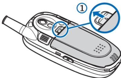
2. Use the side grips (circled) to lift the back cover from the device (2).
