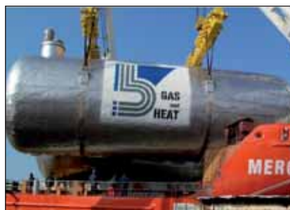
Figure 6 - Type C tank during lifting on board.
