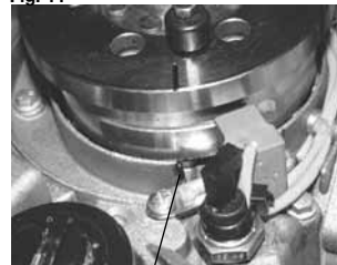
Tacca sul carter Notch on the crankcase Cransur le carter
