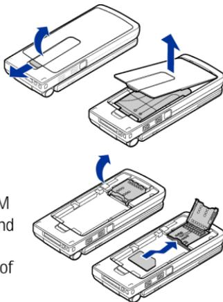
3. Insert the Reduced Size MultiMedia Card (RS-MMC) into the holder's slot. Make sure that the bevelled corner and golden contact area of the RS-MMC are facing downwards.
