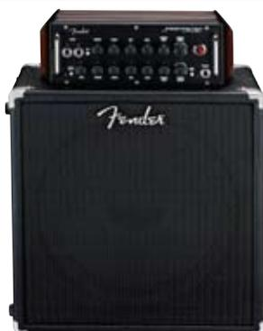
This is the perfect companion enclosure for the JazzMaster Ultralight amp. Features include Italian poplar plywood construction, single 12" Jensen® speaker, magnetic docking system for secure attachment of amp to enclosure, and locking Neutrik® Speakon® speaker connector. Handles 250 watts (at 2 ohms) and only weighs 17 pounds!
