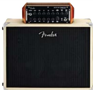
High-quality companion stereo enclosure for the Acoustasonic™ Ultralight amp. Features include Italian poplar plywood construction, internal cabinet divider panel, two 8" Eminence® low-frequency speakers and two high-fidelity 1" dome tweeters, and magnetic docking system for secure attachment of amp to enclosure. Rated at 2x125 watts (stereo) at 4 ohms per side.
