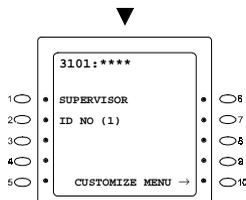
2. The 3101 setting screen appears. Enter the 4-digit ID number and press **HOLD** key to make setting. Each time the **HOLD** key is pressed, the setting changes: 3101→3102→3201.
