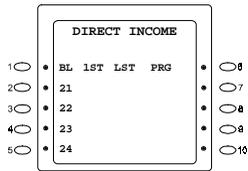
4. Enter the first CO line or private line number using the 10-key pad. (The figure on left shows setting of block No. 03.)
