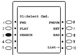
1. Press the **soft** key **1, 2 or 3** or **6, 7 or 8** for the commands to be set, and press the **HOLD** key.
