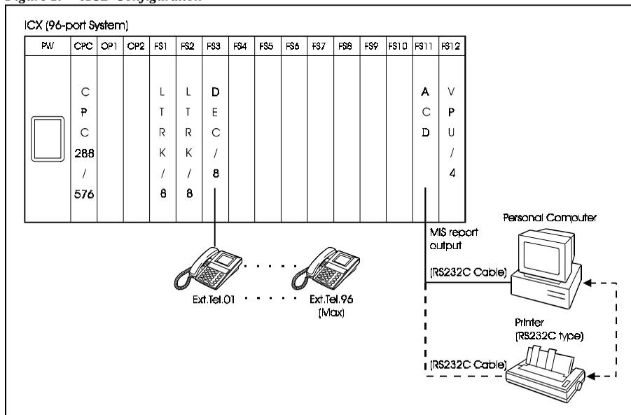
**Note:** Standard RS232C cables cannot be used for connection. Use the special cable included with the ACD card. For PC/printer connecting conditions, see the ACD installation section.
