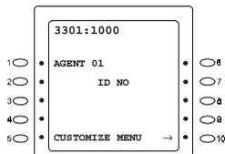
4. Enter 4-digit ID number using the 10-key pad. (The figure on left shows setting of Agent No.01.)
