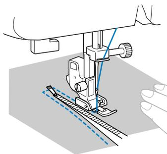
**5** To sew the opposite side of the zipper, release the foot by pressing the button located at the back of the presser foot, fit the zipper foot on the other side of the zipper and continue sewing using the other side notch.
