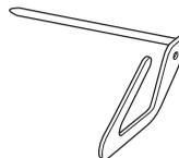
**1** Insert the stem of the quilting guide into the hole at the rear of the walking foot or presser foot holder.
