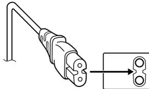
**To avoid electric shock or damage to the unit, first firmly insert the small end of the power cord into the AC Adapter until it is no longer wobbly, and then plug the larger end of the power cord into an AC outlet.**
