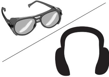
Operating this nailer can propel objects into the air, causing immediate eye damage. To protect yourself, always wear American National Standards Institute (ANSI) approved safety glasses or goggles when operating this equipment. In addition, this nailer discharges at 85-90 decibels. To protect your hearing, always wear ANSI approved ear protection when operating this nailer.
