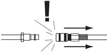
**Always disconnect air from nailer whenever servicing! During maintenance, a nailer connected to air may fire accidentally, causing serious personal injury!**
