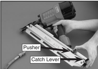
**Figure 3.** Sliding pusher toward the catch lever pusher.
