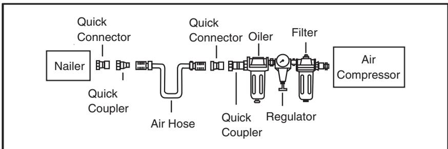
**Figure 2.** Filter/Lubricator/Regulator Unit.
