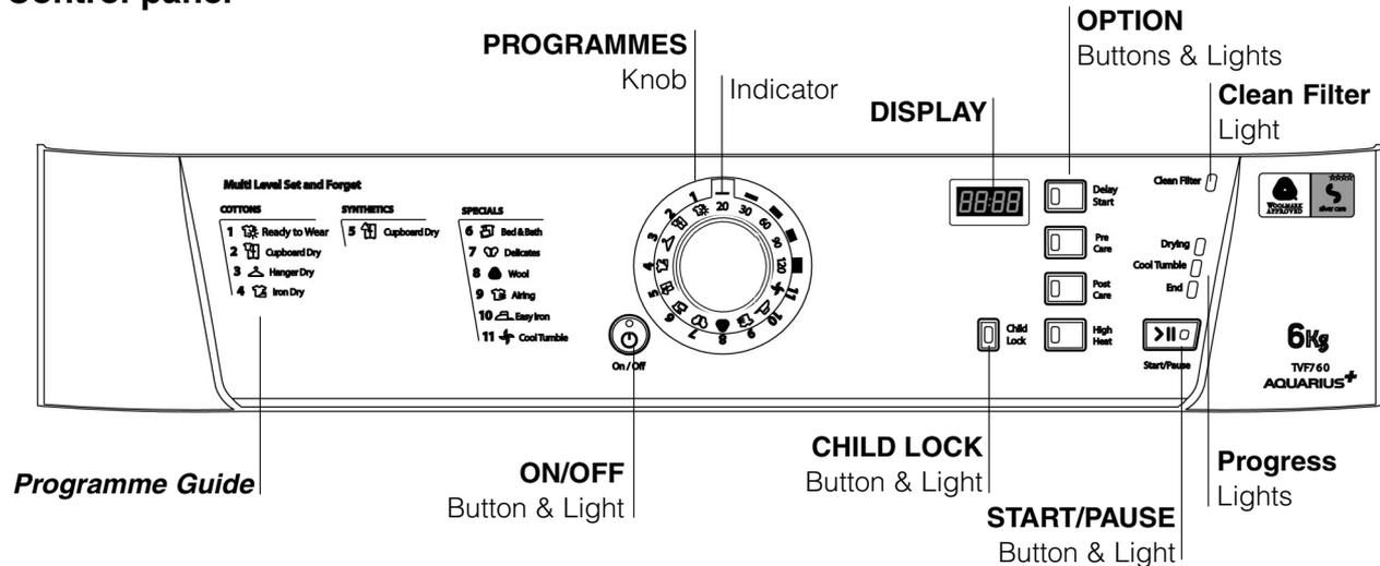
The **ON/OFF** button/light : If the dryer is running and this button is pressed, the dryer is turned off. Press again, the dryer restarts. The light signals that your dryer is in use or ready to select a programme.
