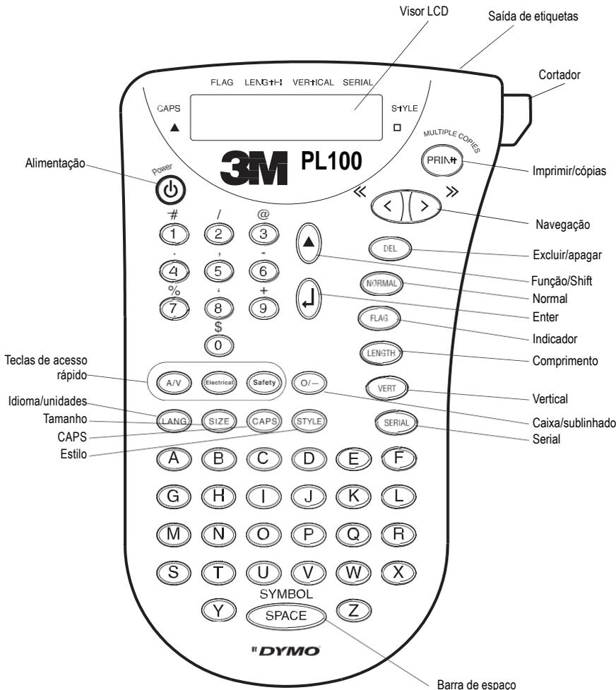
Figura 1 3M™ Portable Labeler PL100
