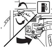
2. Move the choke control located on the engine to "CHOKE" position.
