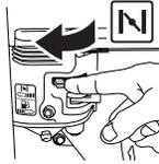
4. Move the ON/OFF switch on engine to the ON position.
