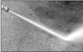
**15° nozzle - Yellow.** This nozzle delivers a powerful 15 degree spray pattern for intense cleaning of small areas. This nozzle should only be used on areas that can withstand the high pressure from this nozzle.
