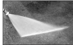
**Chemical nozzle - Black.** This nozzle is used to apply chemicals or cleaning solutions. It has the least powerful stream.
