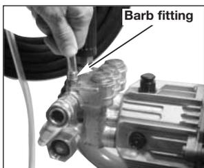
2. Place other end of chemical hose with filter on it into container holding chemical/cleaning solution.
