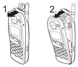
• To replace the cover, first place and close the catches in the lower part of the cover into the corresponding holes in the phone and then gently close the whole cover.
