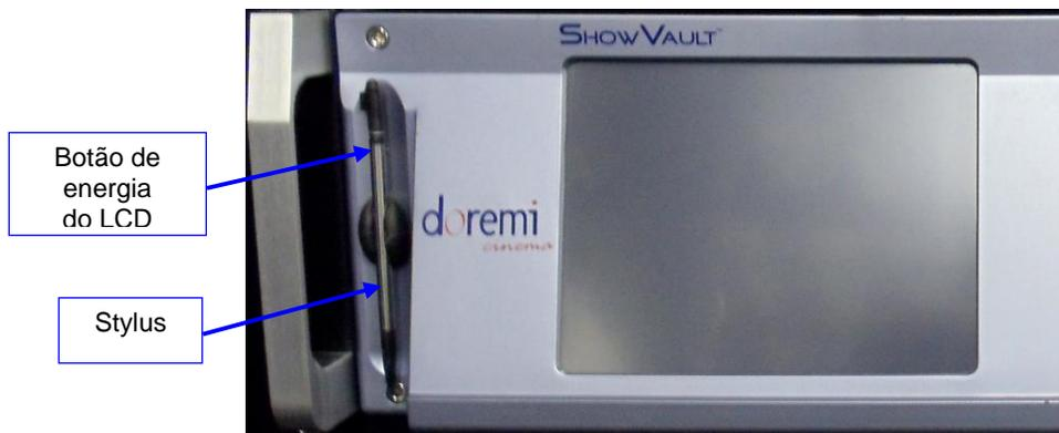
**Figura 6: Tela LCD do painel frontal do ShowVault-3**
