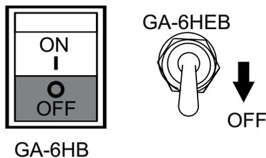
**Figure 18. Idle Control Switch (OFF)**
