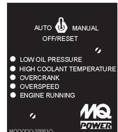
If the engine does not engage (start) by the third attempt, the engine will be shutdown by the engine controller's **Over Crank Protection** mode. If the engine engages at a speed (RPM's) that is not safe, the controller will shutdown the engine by initializing the **Over Speed Protection** mode.
