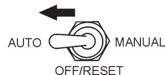
**Figure 53. MPEC Control Switch (AUTO)**
