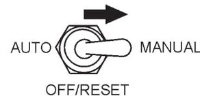
**Figure 39. MPEC Control Switch (Manual Position)**
