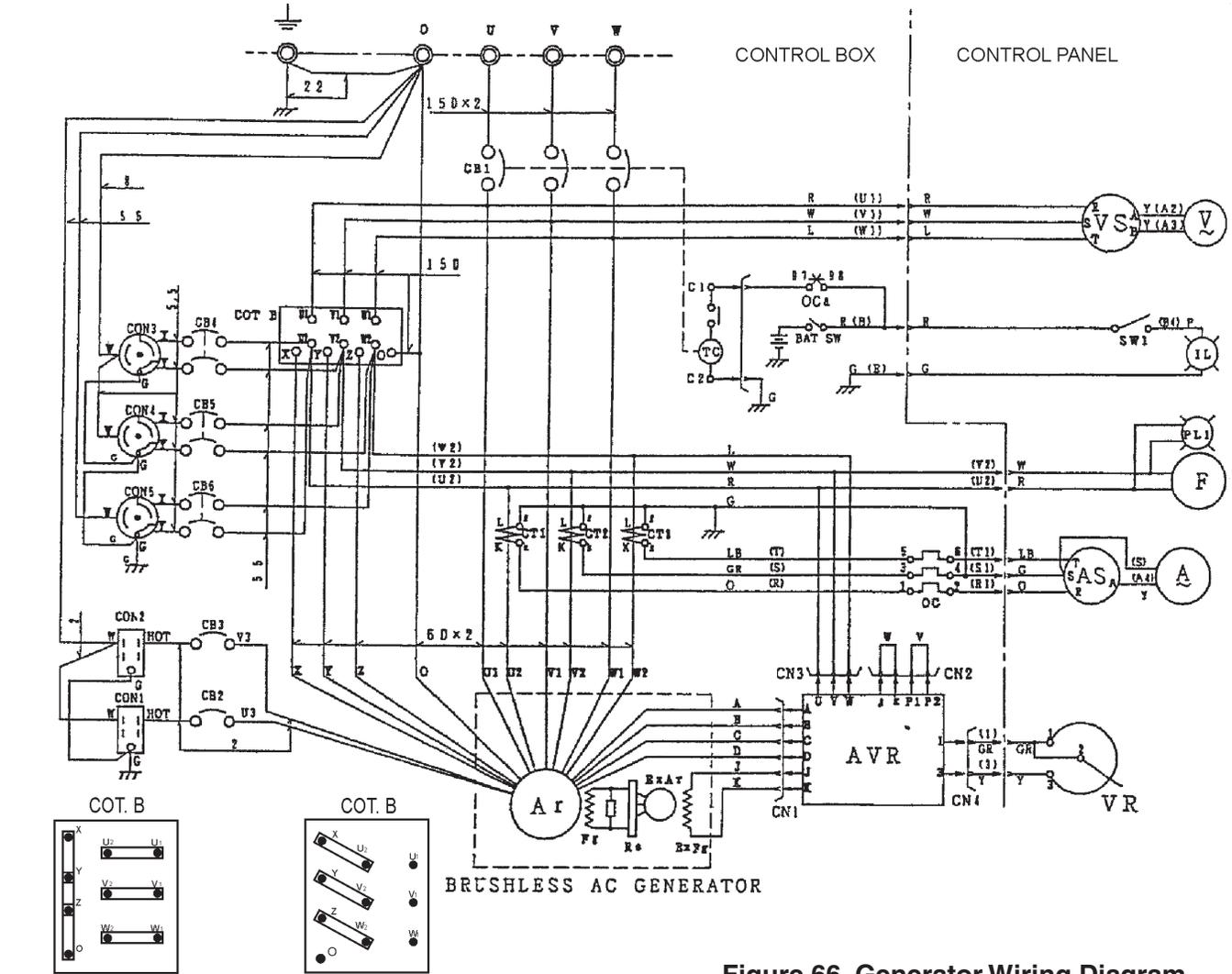
Figure 66. Generator Wiring Diagram
