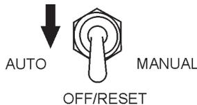
**Figure 55. MPEC Control Switch (Off/Reset)**
