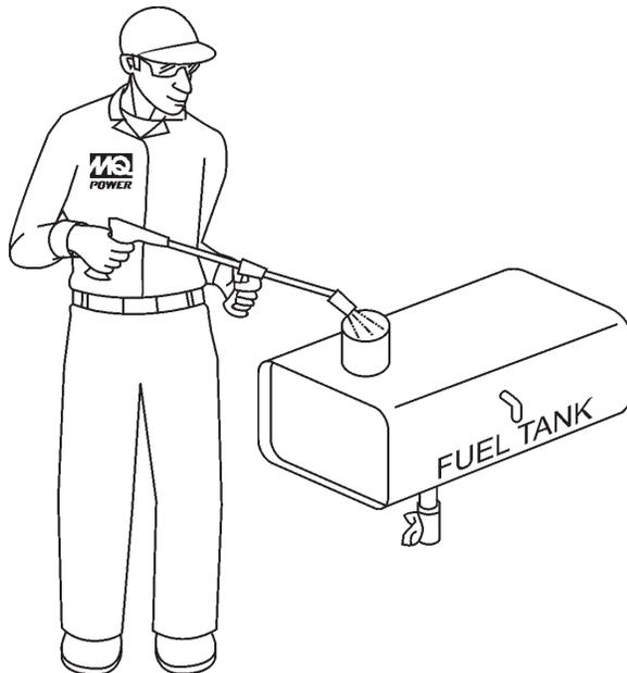
Figure 59. Fuel Tank Cleaning
