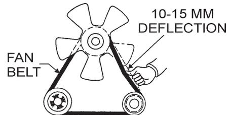
**Figure 18. Fan Belt Tension**
