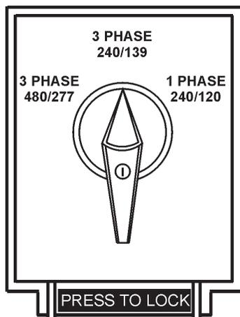
Figure 17. Voltage Selector Switch 240/139V Three Phase Position
