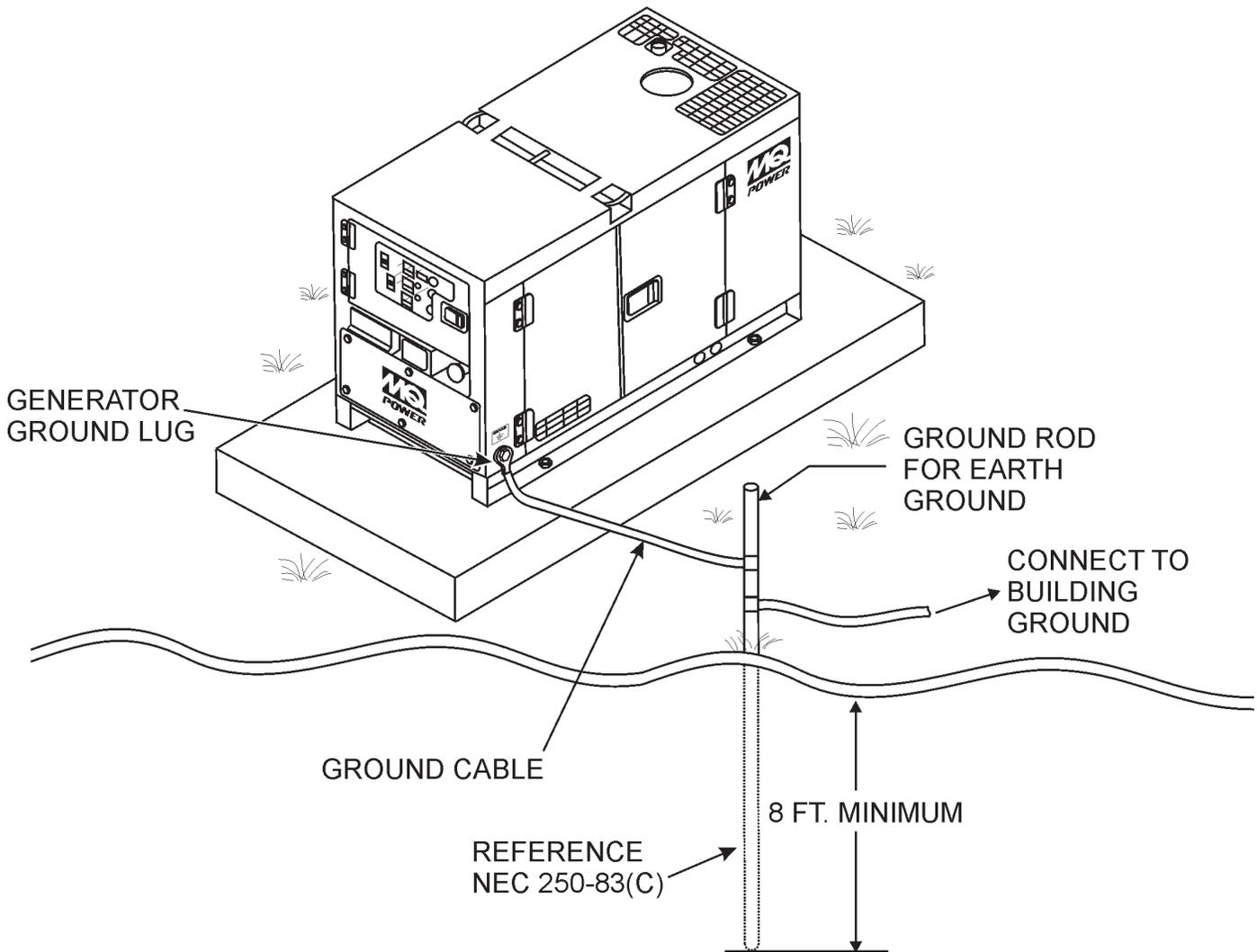
Figure 4. Typical Generator Grounding Application
