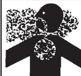
Diesel engine exhaust gases contain poisonous carbon monoxide. This gas is colorless and odorless, and can cause **DEATH** if inhaled. **NEVER** operate this equipment in a confined area or enclosed structure that does not provide ample free flow air.
