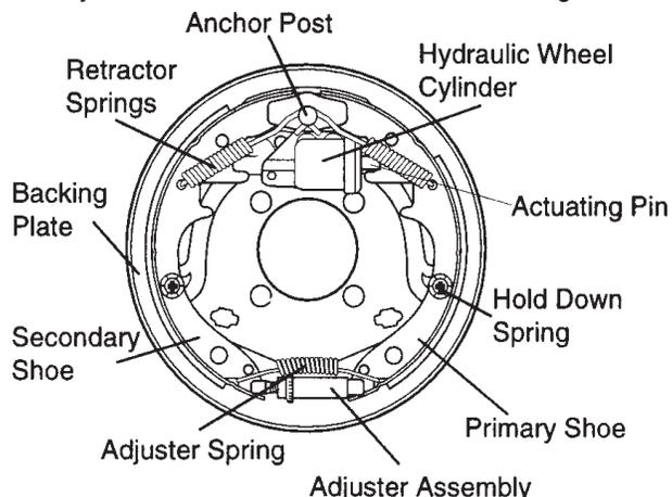
Figure 57. Hydraulic Brake Components
