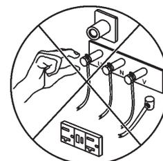
Backfeed to a utility system can cause **electrocution** and or property damage. **DO NOT** connect to any building's electrical system except through an approved device or after building main switch is opened. **ALWAYS** have a licensed electrician perform the installation
