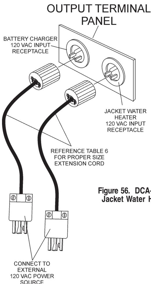
Figure 56. DCA-25SSIU2 Battery Charger & Jacket Water Heater Power Connections
