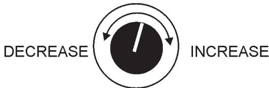
Figure 46. Voltage Adjusted Control Knob
