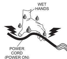
**NEVER** touch output terminals during operation. This is extremely dangerous. **ALWAYS** stop the machine and place the circuit breaker in the **OFF** position when contact with the output terminals is required.
