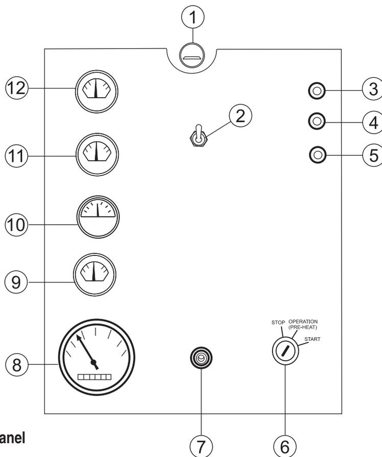
**Figure 7. Engine Operating Panel**
