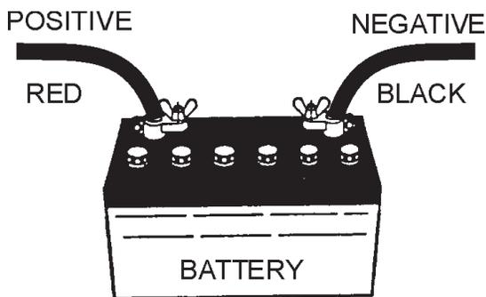
Figure 38. Battery Connections
