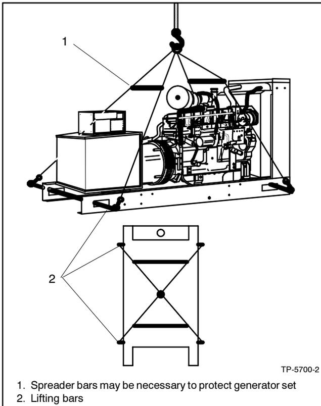
**Figure 2-1** Generator Set with Lifting Bars in Skid
