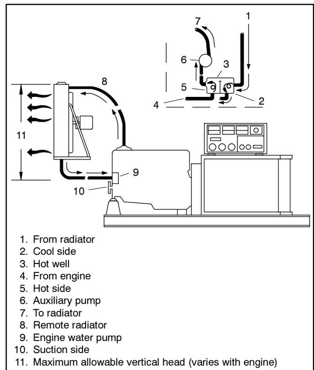
Figure 4-10 Schematic Diagram of Remote Radiator System
