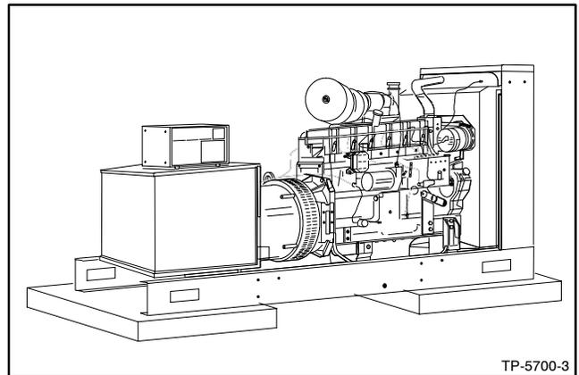
**Figure 3-3** Dual-Pad Mounting
