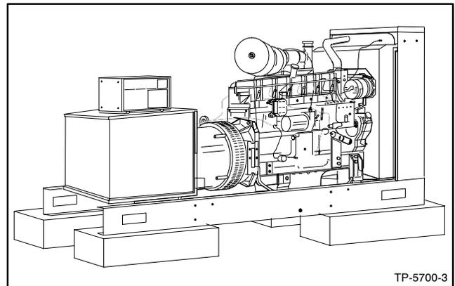
**Figure 3-4** Four-Pad Mounting
