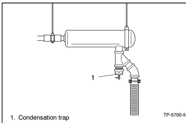
**Figure 5-3** Condensation Trap
