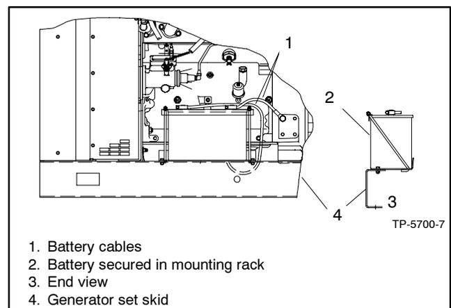
**Figure 7-1** Typical Battery System, Side View
