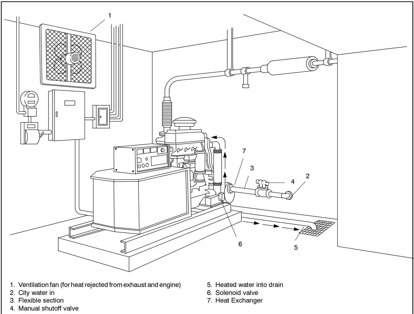
**Figure 4-11** Installation Using City Water Cooling System with Heat Exchanger
