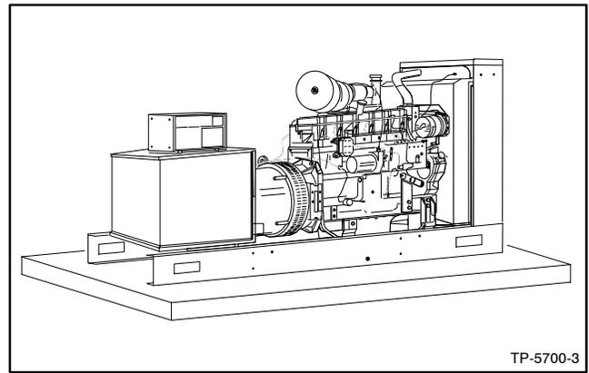
**Figure 3-2** Single-Pad Mounting
