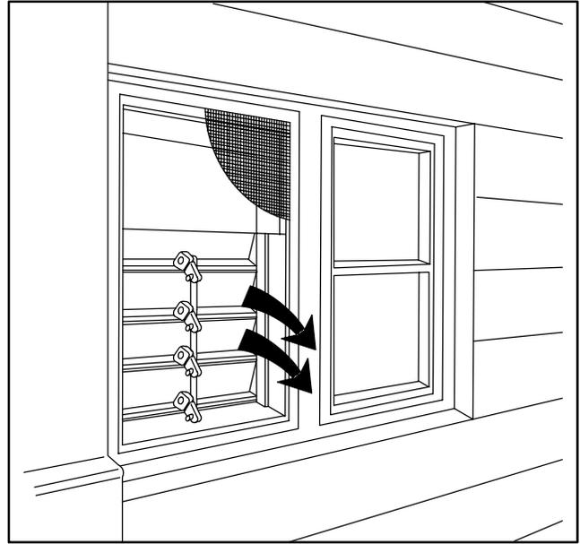
**Figure 4-1** Exhaust Fan-Operated Louvers (fan not shown)
