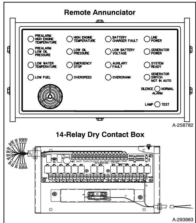
**Figure 7-6** Remote Annunciator with 14-Relay Dry Contact Kit
