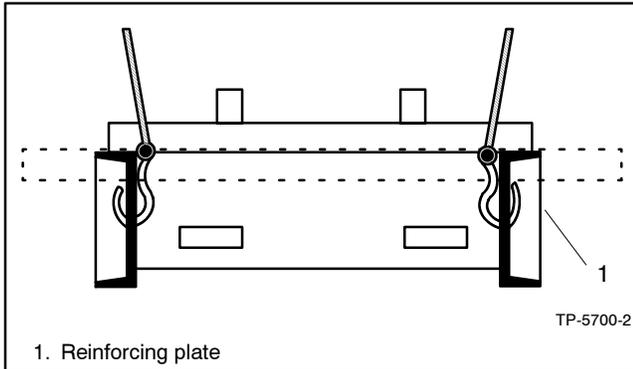
**Figure 2-4** Lifting Hook Placement (above 1000 kW)
