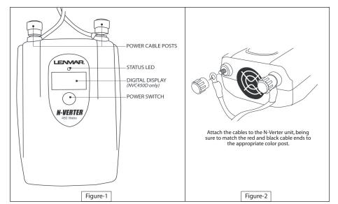
2. If you are using the cigarette lighter adapter, plug it into your vehicle's 12VDC power socket. If you are using the clip leads with the NVC450D, carefully attach them to the vehicle's battery terminals, being very careful not to let the red clip lead touch any metal other than the battery terminal, and also making sure to observe correct polarity (red to red, black to black).
