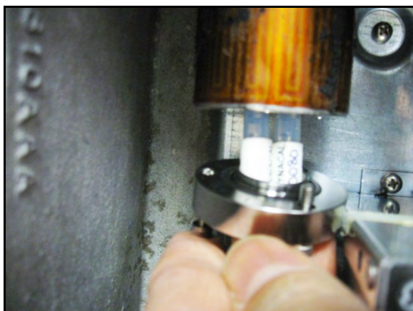
Figura 87: Reinstalar a tampa
