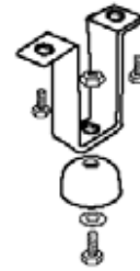
FIGURE 4: Rubber Stopper Attachment to Support Leg
