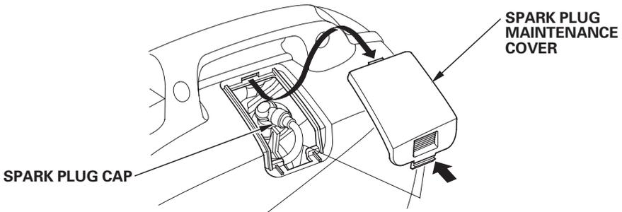
3. Clean any dirt from around the spark plug base.
