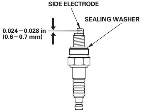
7. Make sure that the spark plug sealing washer is in good condition, and thread the spark plug in by hand to prevent cross-threading.
