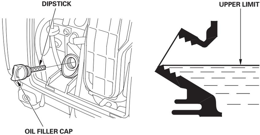
The Oil Alert system will automatically stop the engine before the oil level falls below safe limits. However, to avoid the inconvenience of an unexpected shutdown, check the oil level regularly.
