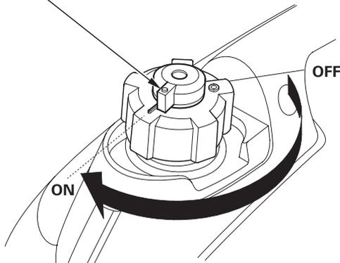
3. Make sure the Eco-Throttle switch is in the OFF position, or more time will be required for warm-up.
