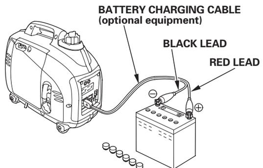
3. Connect the red lead of the battery charging cable to the positive (+) battery terminal and the black lead to the negative (-) battery terminal.
