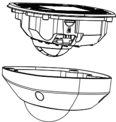
Figure 2-9 Retire a cobertura frontal
