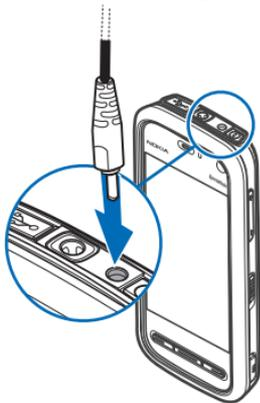
3. When the battery is fully charged, the charging indicator stops scrolling. Disconnect the charger from the device, then from the wall outlet.
