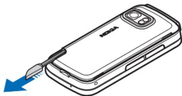
**Important:** Use only a stylus approved by Nokia for use with this device. Using any other stylus may invalidate any warranty applying to the device and may damage the touch screen. Avoid scratching the touch screen. Never use an actual pen or pencil or other sharp objects to write on the touch screen.
