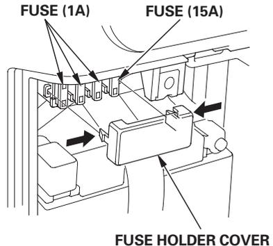
5. Install the fuse holder cover and the battery maintenance cover in the reverse order of removal (see page 56 ).
