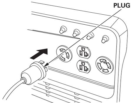
If the generator is overloaded, or if there is a short circuit in a connected appliance, or if the inverter is overheated, the overload indicator (red) will come ON. The overload indicator (red) will stay ON, and after about five seconds, current to the connected appliance(s) will shut off, and the output indicator (green) will go OFF. Stop the engine and investigate the problem.
