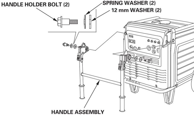
Operation must be checked after attaching a handle.
