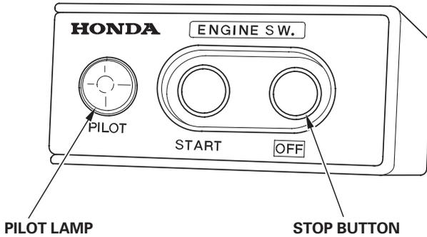
2. Turn the engine switch to the OFF position.
