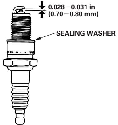
7. Make sure that the spark plug sealing washer is in good condition, and thread the spark plug in by hand prevent cross-threading.
