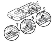
properly inserted and that the golden-colored contact area on the card is facing downwards, and the beveled corner faces upwards.
