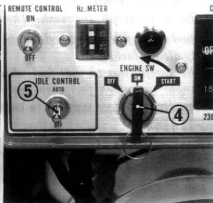
NOTE: When the speed of the starter motor drops after a period of time, it is an indication that the battery should be recharged.
