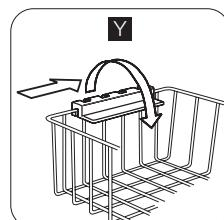
Turn and fix the handles for these two positions as shown in the picture.
