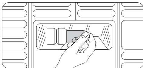
2. Replace the lamp with one of the same power and specifically designed for household appliances. (the maximum power is shown on the lamp cover)
