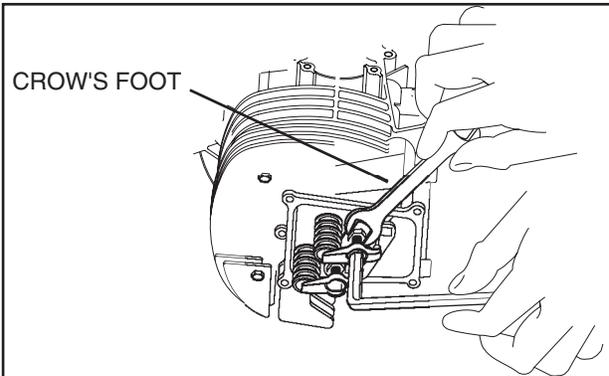
Figure 6-52 – Tightening the Jam Nut
