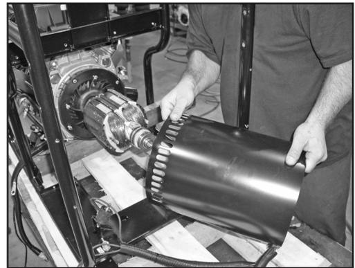
Figure 7-8. – Remove Stator
