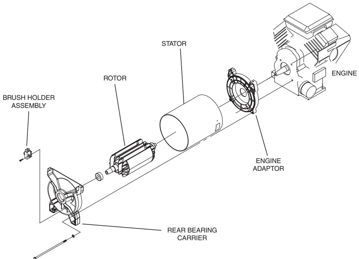
*Figure 3-1. – AC Generator Exploded View*
