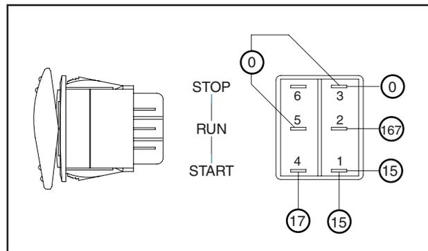
Figure 6-36. – Start-Run-Stop Switch (SW1)
