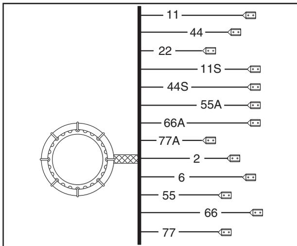
Figure 3-9. – Stator Winding Leads
