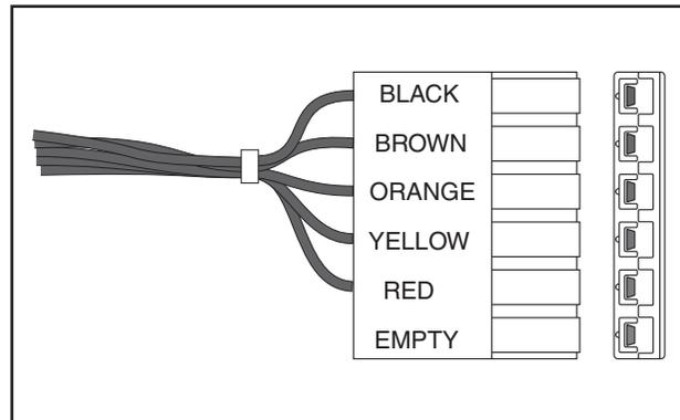
Figure 6-4. – Six Pin Connector Wire Colors
