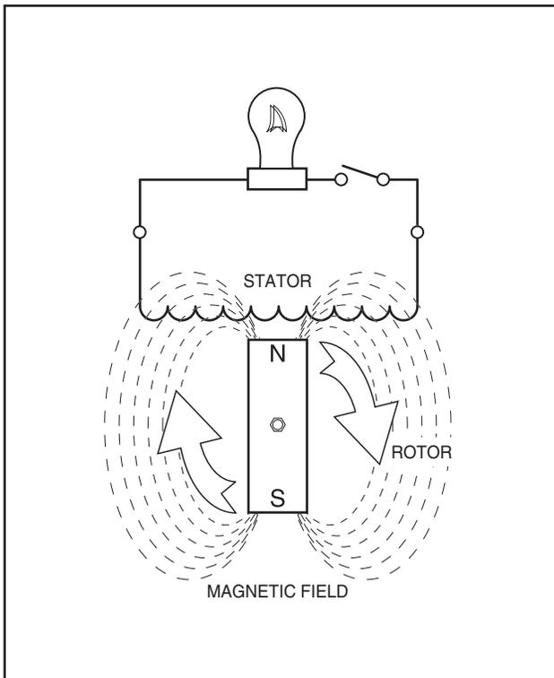
Figure 1-4. – A Simple AC Generator
