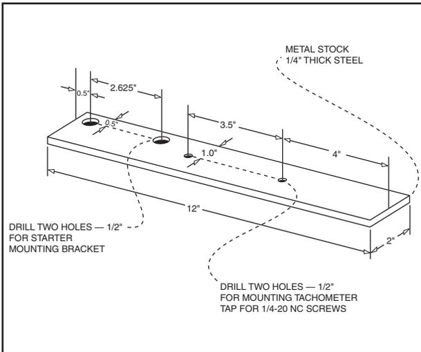
Figure 6-33. – Test Bracket Dimensions
