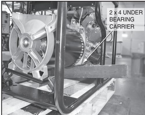
Figure 7-6. – Support Alternator
