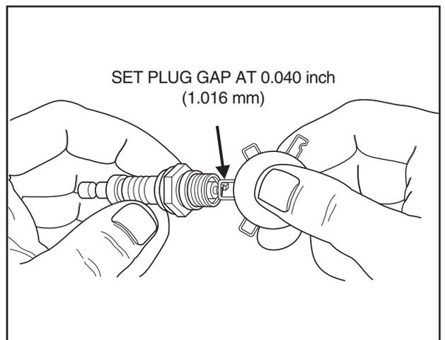
*Figure 6-39. – Setting Spark Plug Gap*
