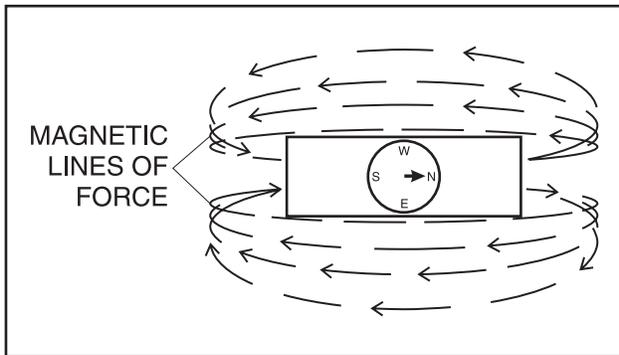
Figure 1-1. – Magnetic Lines of Force
