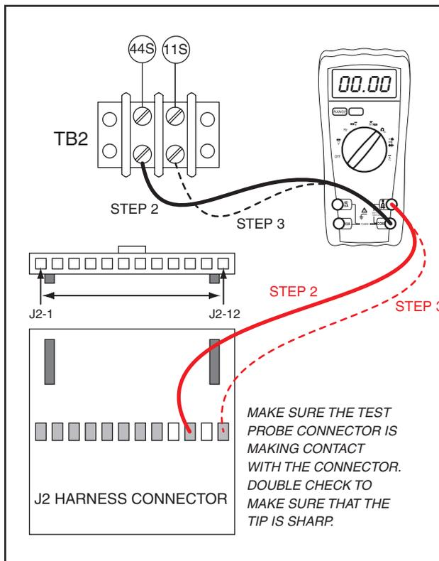
Figure 6-58. – Check Wires 11S & 44S
