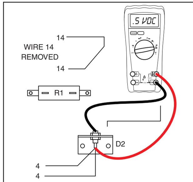
Figure 6-16. – Diode Test Step 6
