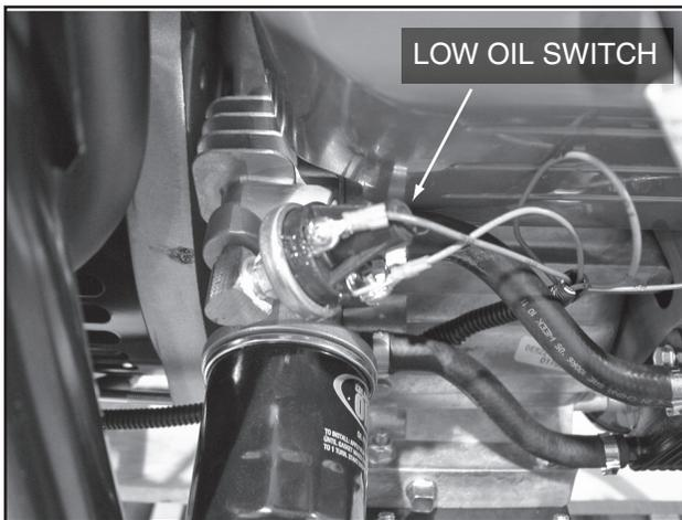
Figure 6-53. – Low Oil Pressure Switch
