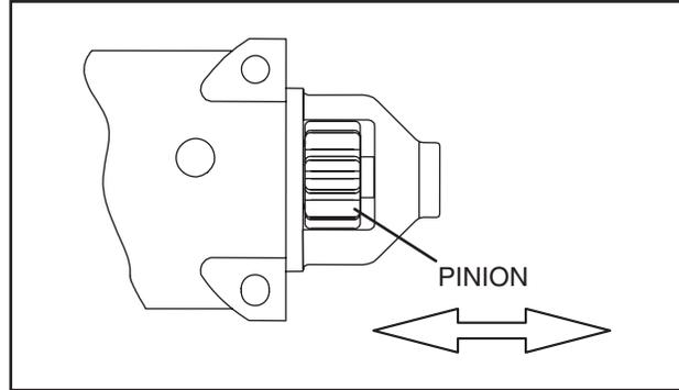
Figure 6-30. – Check Pinion Gear Operation
