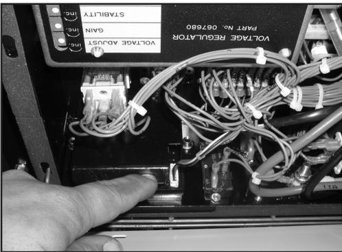
Figure 7-2. – Stepper Motor Harness
