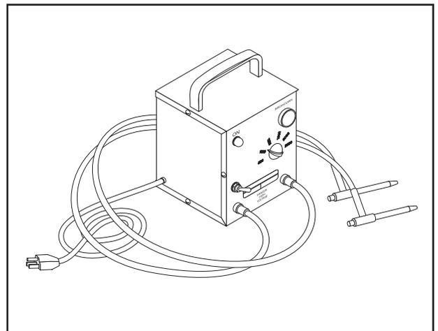
Figure 3-8. – One Type of Hi-Pot Tester
