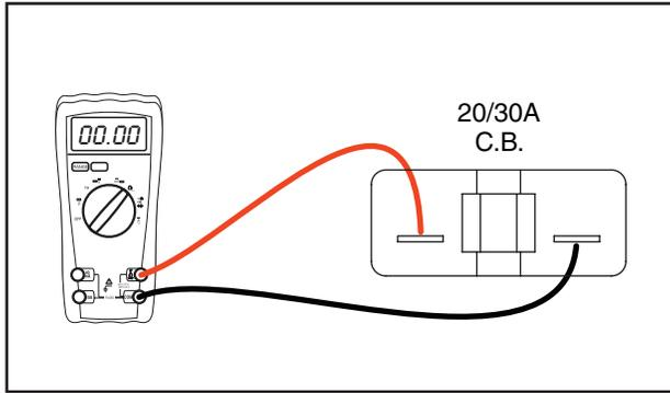
Figure 6-8. – 20/30 Amp Breaker Test Points
