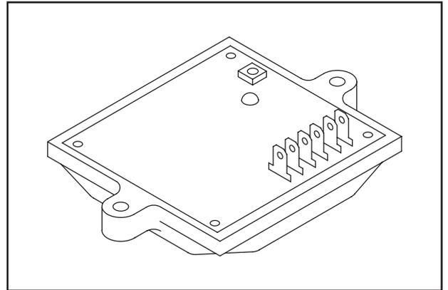
Figure 3-7. – Typical Voltage Regulator Found on 17.5 kW Units
