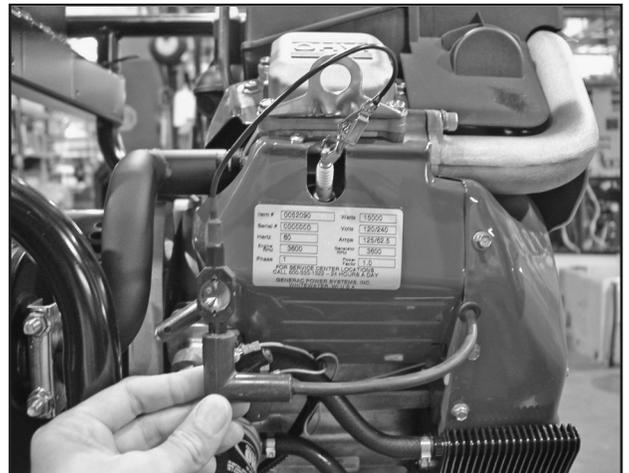
*Figure 6-38. – Checking Engine Miss*
