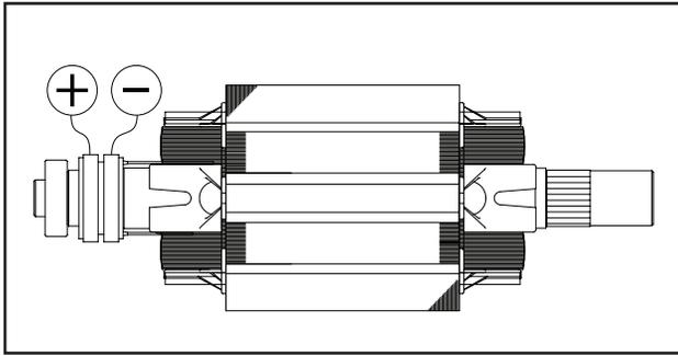
Figure 3-2. – The 2-Pole Rotor Assembly
