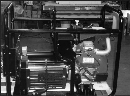
Figure 7-1. – Fuel Tank Removed
