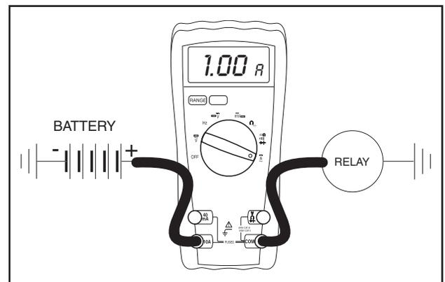
*Figure 2-4. – A VOM as an In-line meter*
