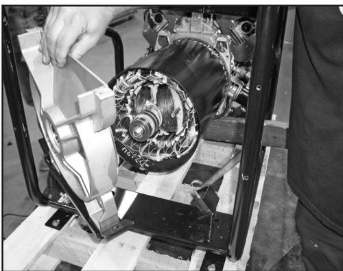
Figure 7-7. – Remove Bearing Carrier
