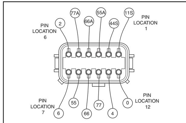
Figure 3-10. – C1 Connector Pin Location Numbers (Female Side, Located to the Right When Facing the Control Panel)
