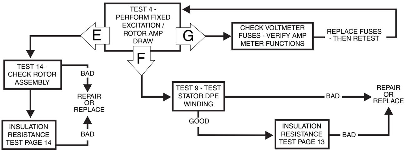
**Problem 3 - Excessive Voltage/Frequency Droop When Load is Applied**
