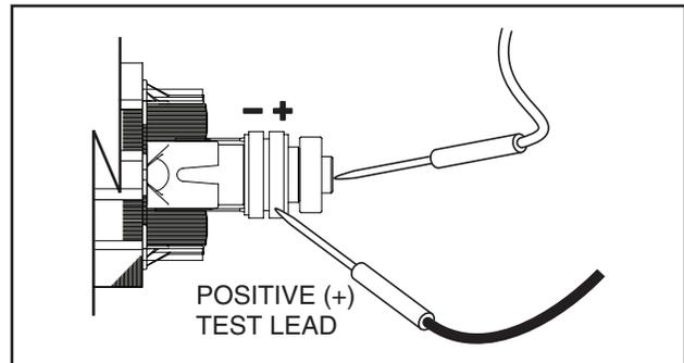
Figure 6-22. – Testing at Slip Rings
