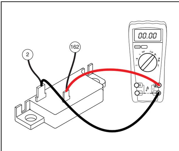
Figure 6-9. - Testing Excitation Circuit Breaker
