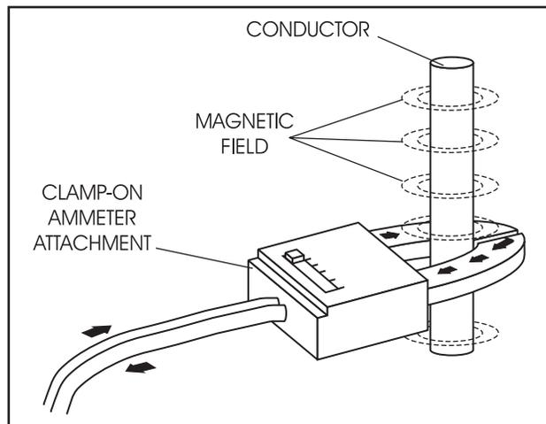
Figure 6-31. – Clamp-On Ammeter
