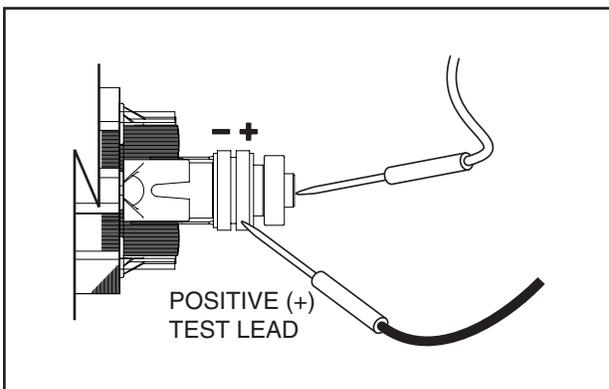
*Figure 3-10. – Testing Rotor Insulation*
