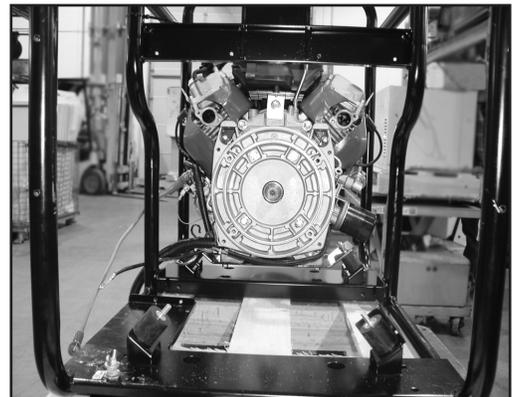
Figure 7-10. – Engine Ready for Removal
