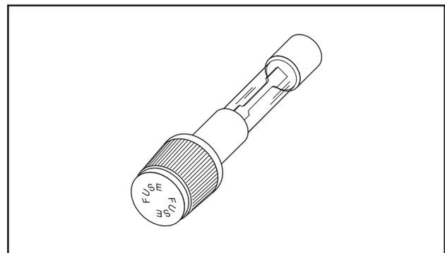
Figure 6-27. – 10 Amp Fuse (Located in Rear of Control Panel)
