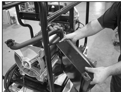
Figure 7-5. – Remove Muffler
