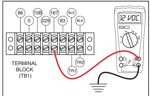
Figure 6-45. – Test Wire 167, Step 3
