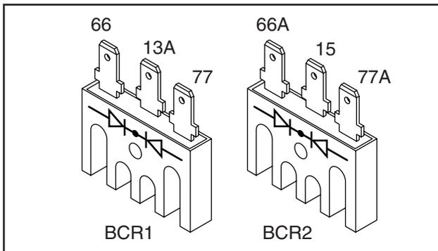
Figure 6-25. – Battery Charge Rectifier
