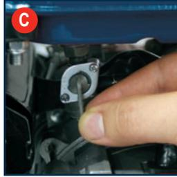
2. Turn the fuel valve (20) clockwise to the 'on' position (Fig. C).
