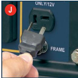
**Note.** This usage is applicable for charging only 12V batteries. Only use the DC plug (19) to charge lead acid type batteries. DO NOT charge Nicad or any other type of batteries.
