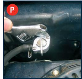
**Note.** This filter can be cleaned in petrol to remove any build-up of dirt on the outside of the filter, or the filter can be replaced. Do not operate the generator without this filter in place. To replace the filter after cleaning, or with a new filter, simply screw the filter into the inlet side of the tap.
