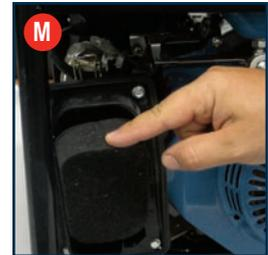
**IMPORTANT.** Never run the engine without the air filter element in place.
