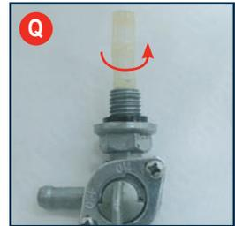
5. Ensuring the small seal is fitted to the tap thread, screw the tap back into the tank by a FULL 3–4 turns. Orientate the tap so the outlet of the tap is towards the rear of the tank, and the tap control is to the right hand side of the tank. Holding the tap firm, tighten the lock nut, ensuring the seal is clamped between the lock nut and the tank (Fig. R).
