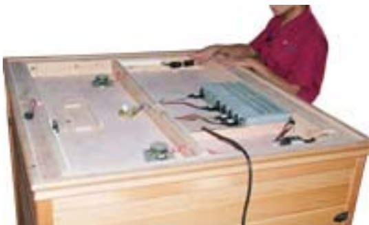
FIG-18 Connectors on the external top board
