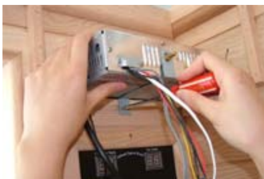
FIG-15.2 Fix the CD to the metal support
