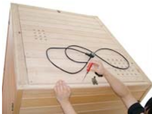
FIG-26 Fix the external board with screw
