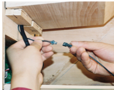
FIG-21 Link the sensor connectors
