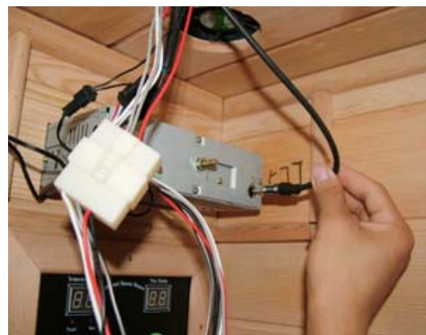
FIG-23 link the antenna connectors
