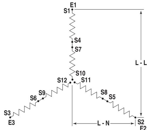
Figure 7.3 — Stator Power Winding Connections - 3-phase, 120/208V (12 Lead)
