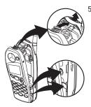
5 Place the bottom of the cover against the bottom of the phone. Make sure all three sets of plastic tabs line up with their respective slots, as shown at left. Close the cover and snap it shut all the way around the edge of the phone.
