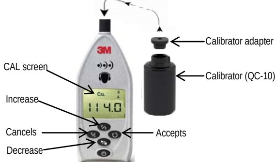
Figure 1-10: Calibrating the SD-200
