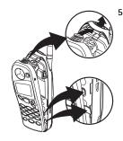
Place the bottom of the cover against the bottom of the phone. Make sure all three sets of plastic tabs line up with their respective slots, as shown at left. Close the cover and snap it shut all the way around the edge of the phone.
