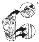
6 Place the bottom of the cover against the bottom of the phone. Make sure all three sets of plastic tabs line up with their respective slots, as shown at left. Close the cover and snap it shut all the way around the edge of the phone.
