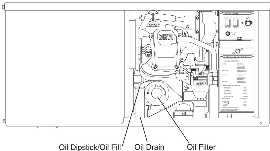
9. Install and tighten the oil fill cap and the dipstick before operating the engine.
