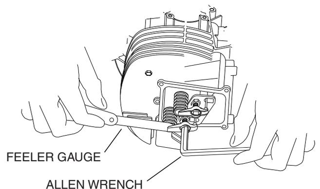
2. When valve clearance is correct, hold the pivot ball stud with the allen wrench and tighten the rocker arm jam nut with a crows foot. Tighten the jam nut to 65-85 inch-pounds torque. After tightening the jam nut, recheck valve clearance to make sure it did not change (Figure 3.8).
