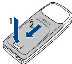
2. To remove the front cover, gently prise the back part of the phone away from the front cover beginning at the bottom of the phone.
