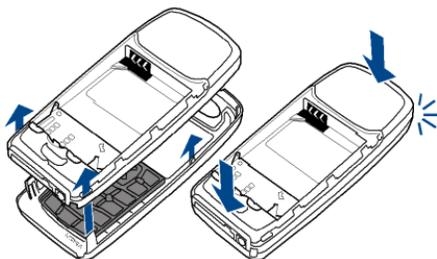
5. Place the back cover and the phone properly together (1) and slide the back cover into its place (2) until the back cover release button is properly locked.
