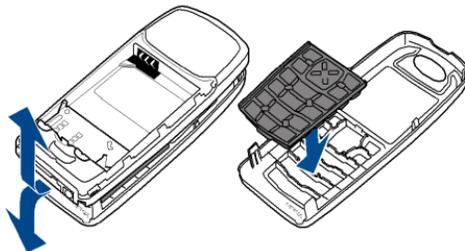
4. To attach the front cover, first place the phone and the front cover properly together and then gently push on t the top of the phone until the catch is locked properly.
