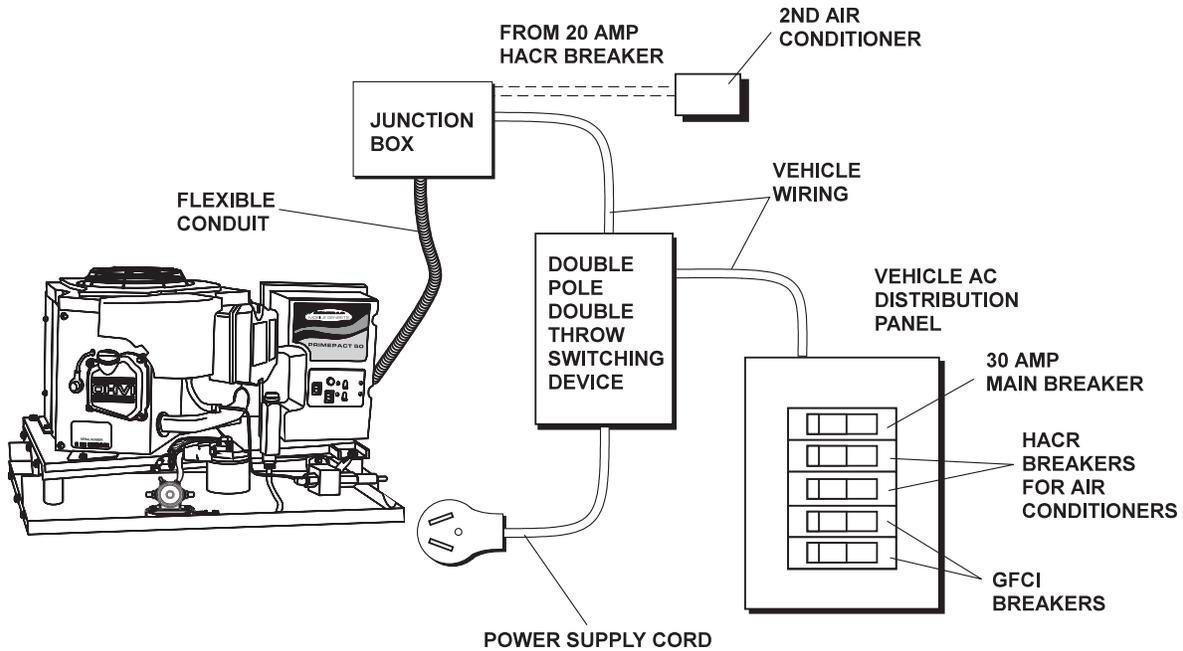
Figure 2.19 – Installation With Isolation Receptacle
