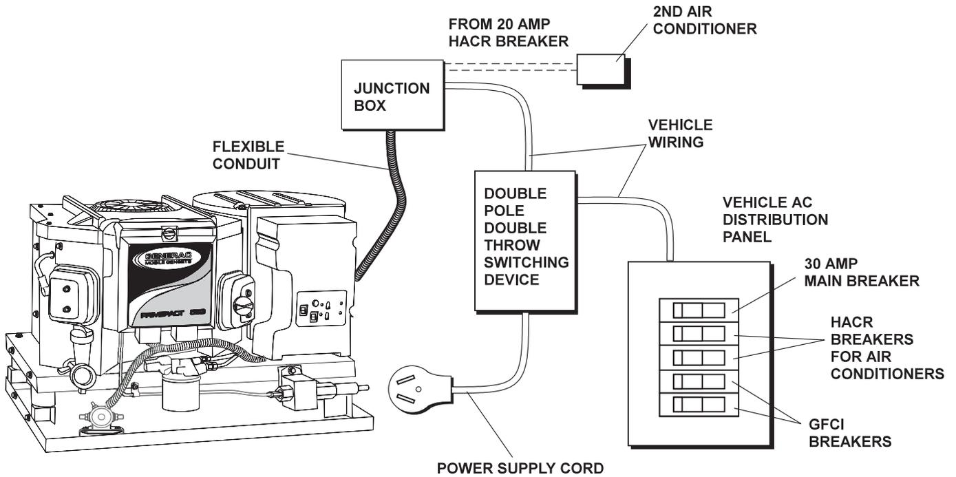
Figure 2.19 — Installation With Isolation Receptacle
