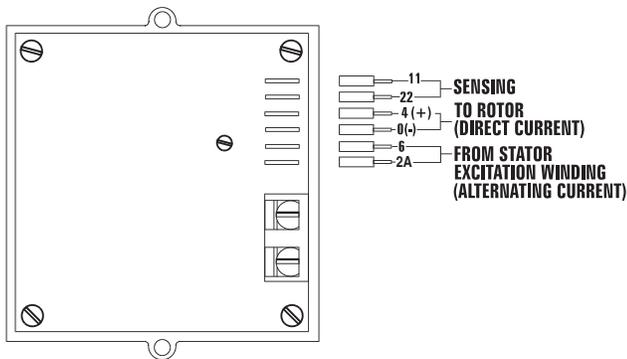
The voltage regulator also incorporates a “voltage surge protection circuit.” This circuit prevents troublesome surges in the generator AC output voltage. Voltage surge is a common cause of damage to electronic equipment.
