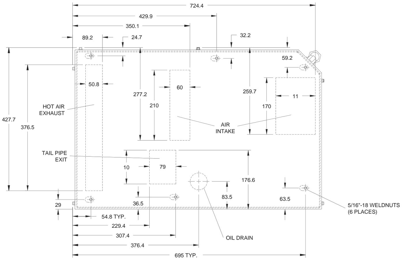
All measurements are in millimeters, 25.4 mm = 1".
