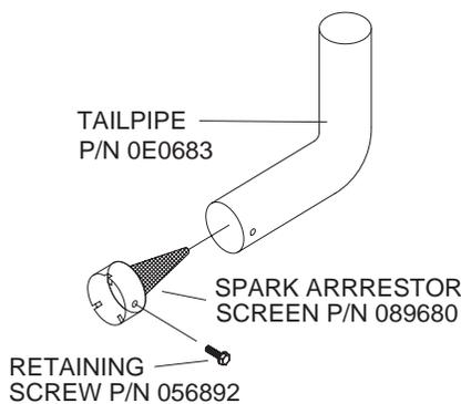
Figure 2.12 — Spark Arrester Installation
