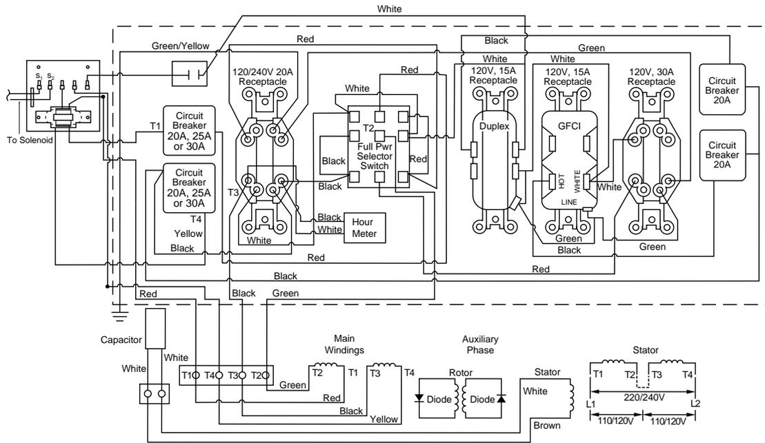
Figure 33 - Wiring Diagram, Model RGH550AIE
