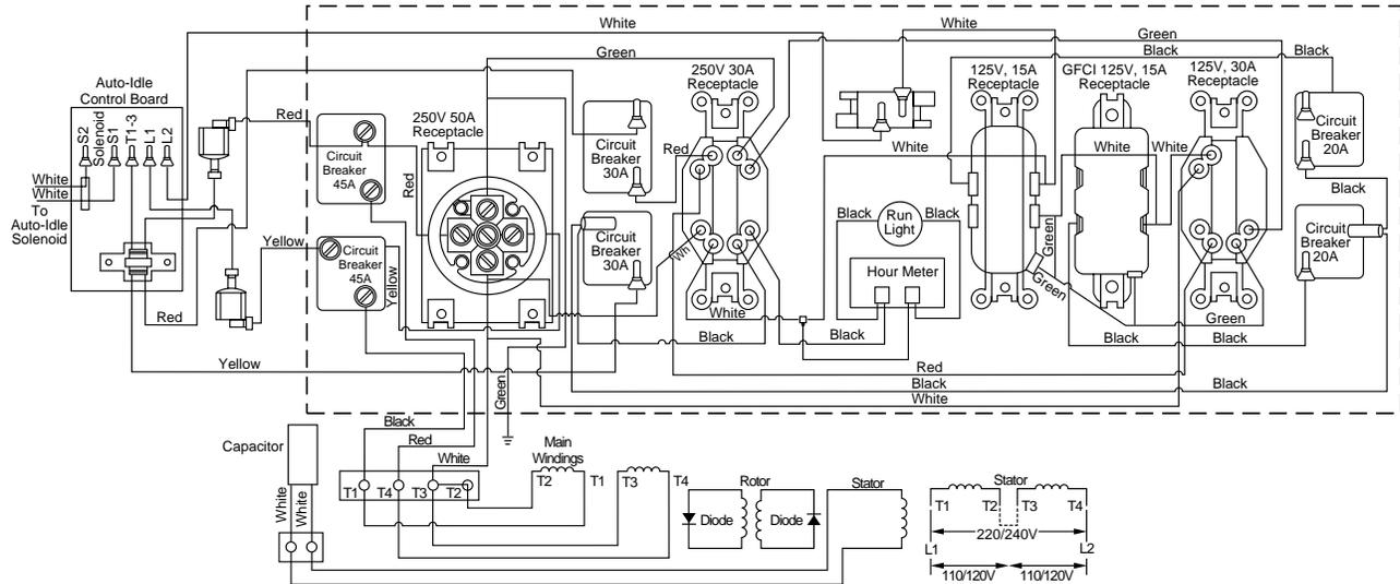
Figure 35 - Wiring Diagram, Model RGH11000AIE
