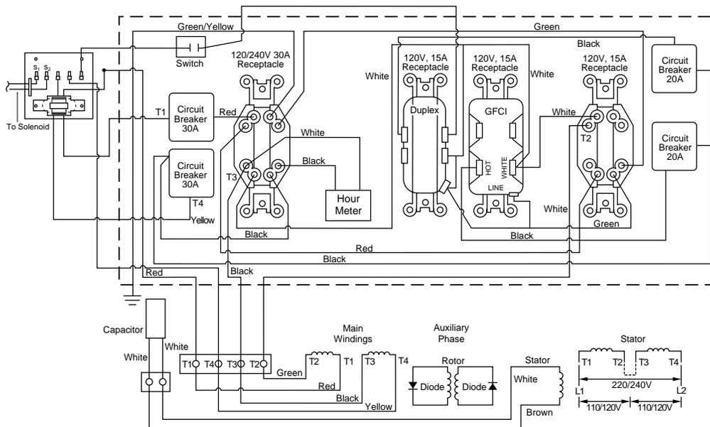
Figure 34 - Wiring Diagram, Model RGH750AIE
