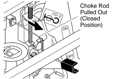
**Figure 20 - Choke Rod Closed (Model RGH3000PR Only)**
