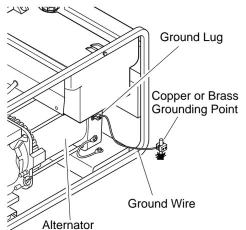
**Figure 16 - Grounding Generator (Model RGH5500A Shown)**
